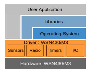
Figure 3: Software Architecture
